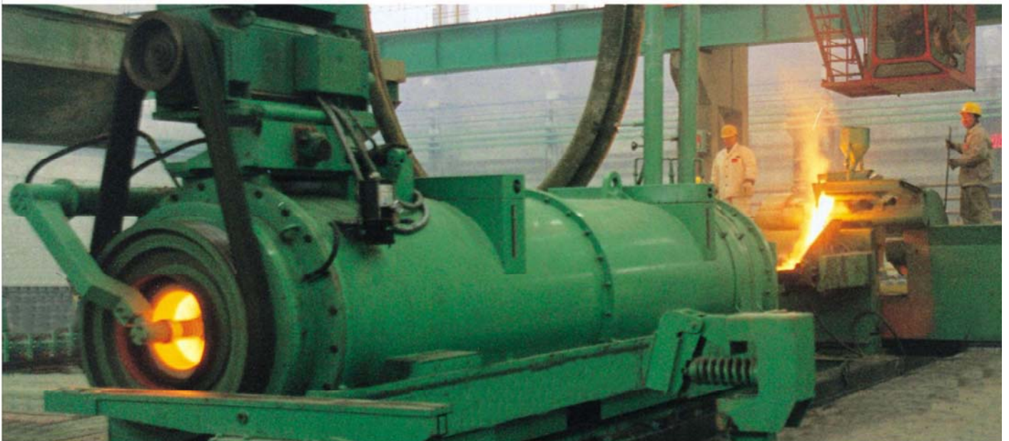
离心浇铸 Centrifugal casting
