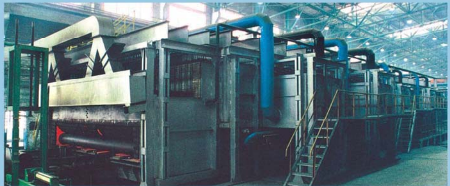
60米退火炉 60m annealing furnace
