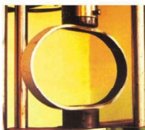
压环试验 Hardness test
