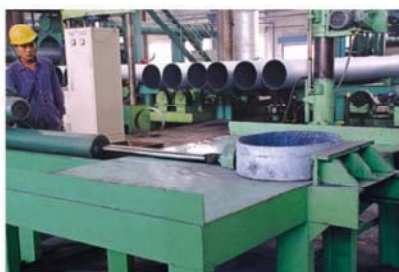
压扁试验 Flat-pressing test
