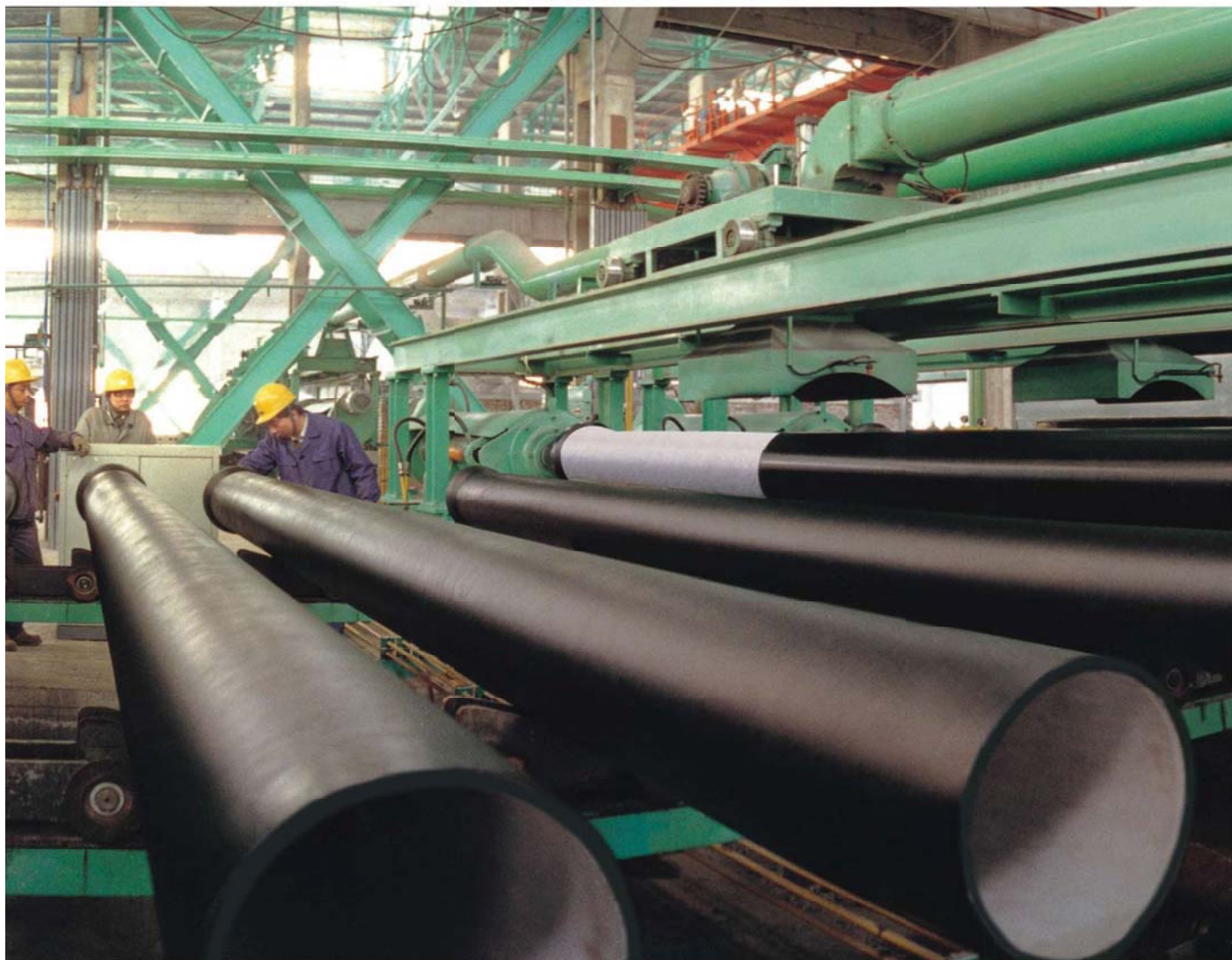
沥青喷涂 Bitumen coating
