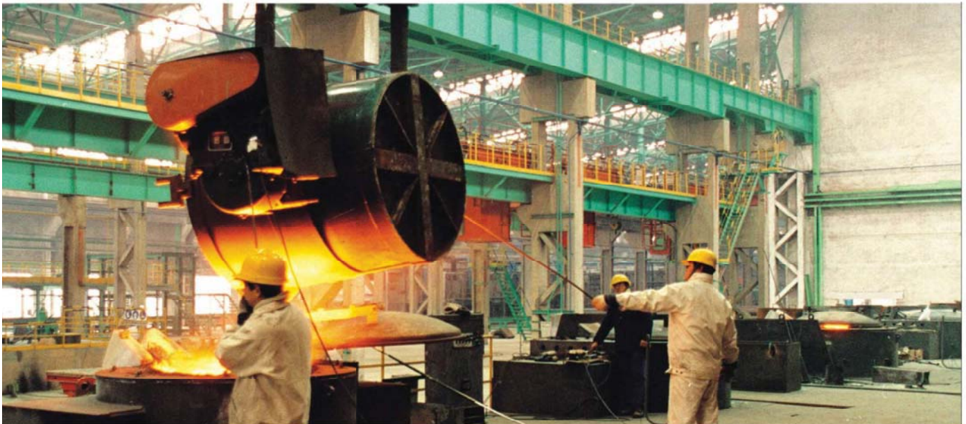
电炉升温及调质 Heating and sphereodization in induction furnace
